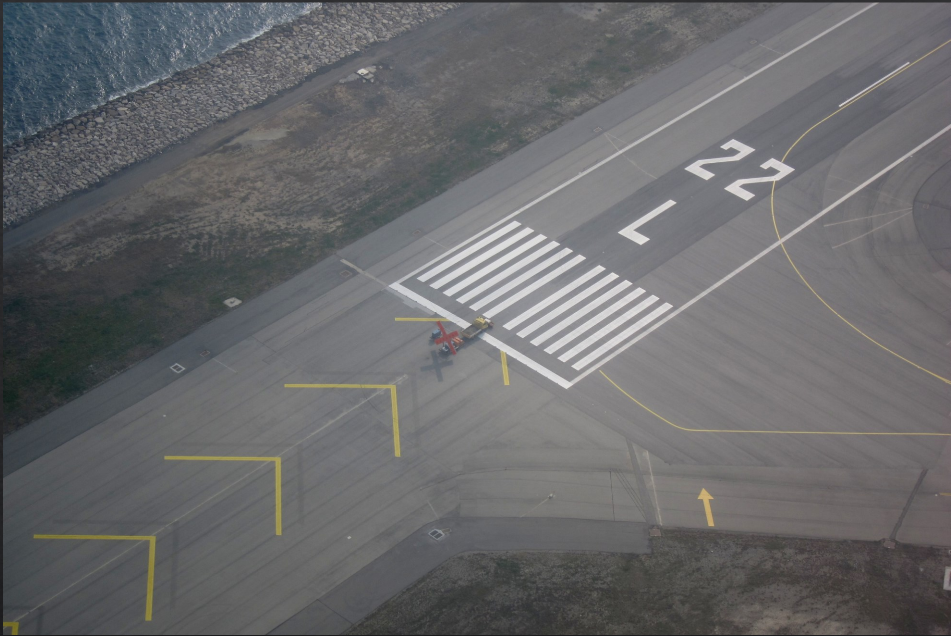
Olivier Cleynen : Threshold of the 22L runway at Nice Airport (NCE), closed for maintenance on that day.
