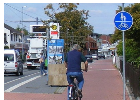
Abbildung 7: highway=path foot=designated bicycle=designated segregated=no surface=paving_stones
