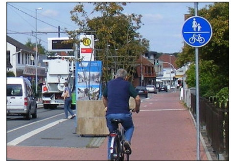
Abbildung 7: highway=path foot=designated bicycle=designated segregated=no surface=paving_stones
